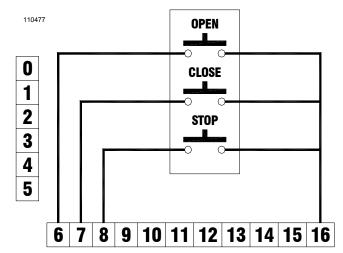
Figure 17: Wiring 3-Button Station
